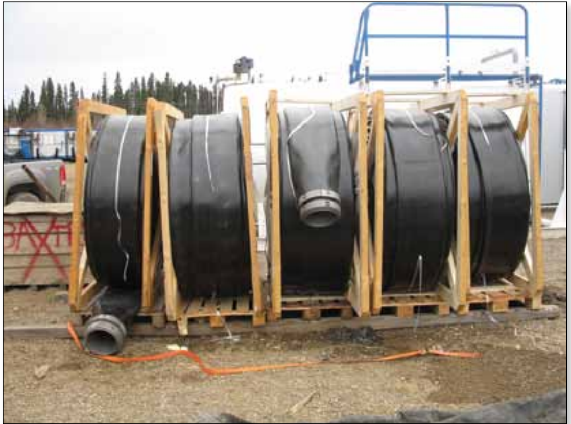
1,000m x 10" MINEFLEX Delivered into the field
