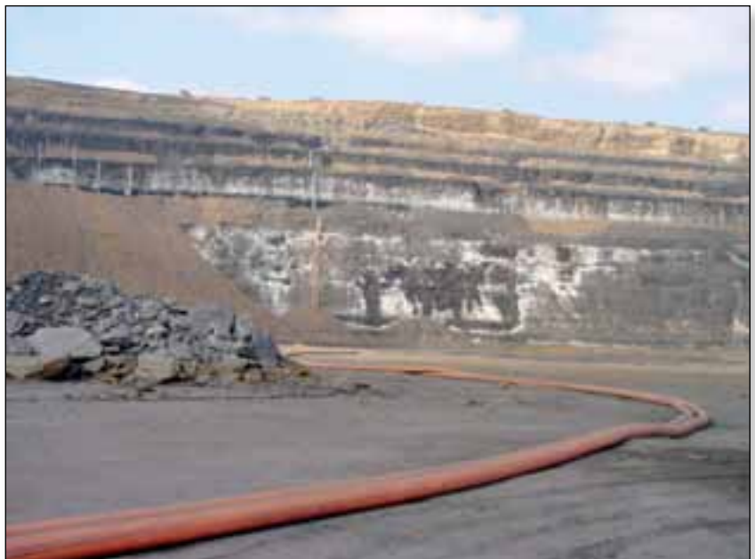
High pressure dewatering
